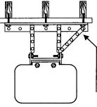
For finished ceilings, or if structural beams are out of position for mounting, use a third mounting angle making sure it is securely mounted to beams.
